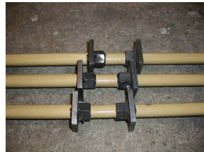
Photo 1 Fixing plates of de-bonded vertical rebar
