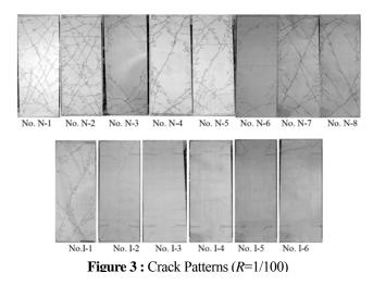
have pinching phenomenon at the occurrence of large deformation after R = 1/67. This seems to be caused by the axial bars that work as bending bars. In the relation of #I-2 at the second R = 1/40 cycle, the load dropped because one of the X bars fractured at the welded part. These bars of specimens #I-2 and 3 were quench-hardened for strengthening, and weldability was not good.
